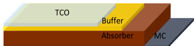
Fig. 1. Structure of the p-n heterojunction solar cell based on CdS/SnSe.
